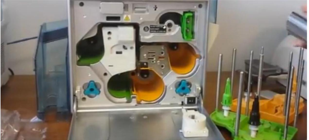
When installing a used ink ribbon, align the yellow side of the unused ribbon with the arrow indicated on the label of the cassette. If the position of the yellow side is not properly aligned, the print may turn out light.
