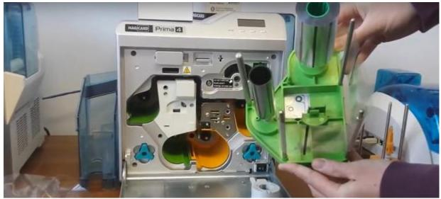
**Step 2:** Insert the cassette all the way in along the guide rail until a "click" sound is heard. Close the printer door.
