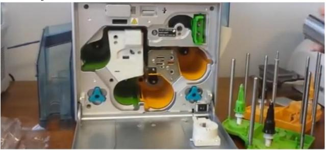
When installing a used ink ribbon, align the yellow side of the unused ribbon with the arrow indicated on the label of the cassette. If the position of the yellow side is not properly aligned, the print may turn out light.
