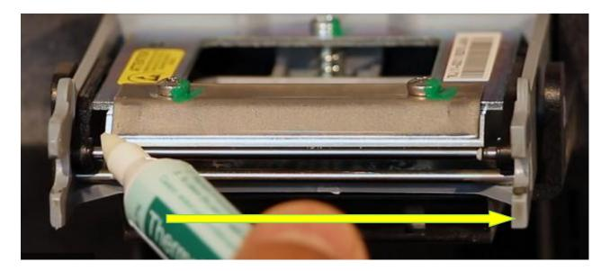
Always clean the printer head in one direction not moving the thermal printer cleaning pen forth and back.
