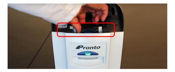
Remove the metal bar from the sticky roller and keep it in a safe place. Every new ribbon will come along with the new
