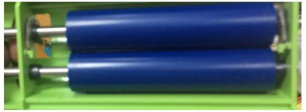
After cleaning dry the rollers make sure no wet or liquid crystals are left on the rollers then fix back in the printer.
