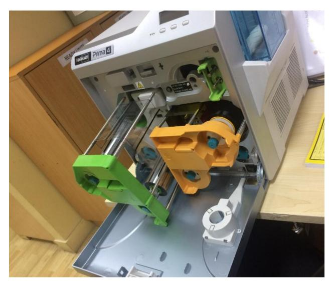
Remove cards as well from the input hopper.
