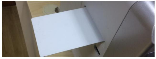
Repeat this process for at least five minutes to make sure dirty parts inside the printer rollers are removed.
