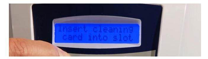
With your new cleaning card open select yes on the printer and insert the cleaning card from the front.
