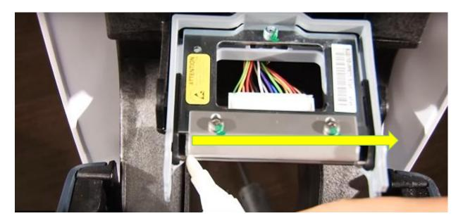
Always clean the printer head in one direction not moving the thermal printer cleaning pen forth and back.
