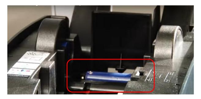
Remove the metal bar from the sticky roller and keep it in a safe place. Every new ribbon will come along with the new
