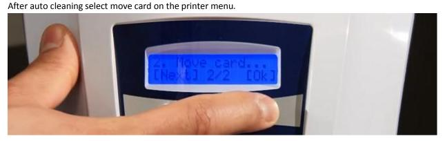
Fold the card and place it on the main roller press move forward for about 15 seconds then press back also wait for at least 15 seconds.
