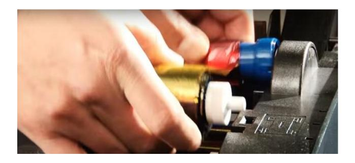
Remove the blue sticky roller from the printer is located towards the back side of the printer.
