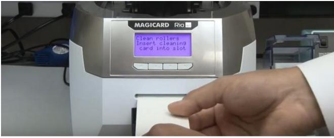
With your new cleaning card open select yes on the printer and insert the cleaning card from the front.
