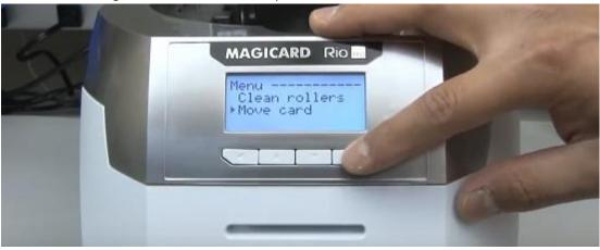
Fold the card and place it on the main roller press move forward for about 15 seconds then press back also wait for at least 15 seconds.
