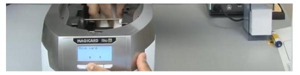
After this process you may also wish to clean the back side of the printer card feeding roller.
